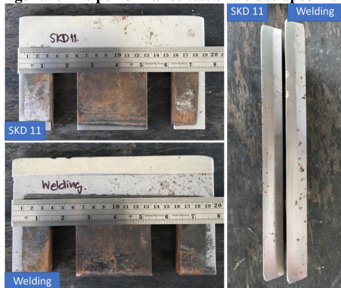
Figure 10. The crusher blade after chopping plastic
